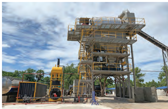
Linnhoff CMX1500 CompactMix asphalt plant is equipped with the energy-saving double screen drum technology.
