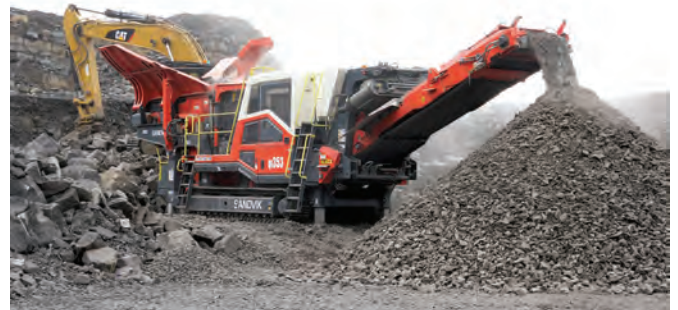
ALL IMAGES: The new Sandvik QI353 mobile crusher is targeted at quarry, recycling and contractor segments.
