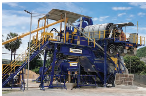
Linnhoff TSD1500 MobileMix asphalt plant features fully integrated four basic mobile modules with built-in chassis.
