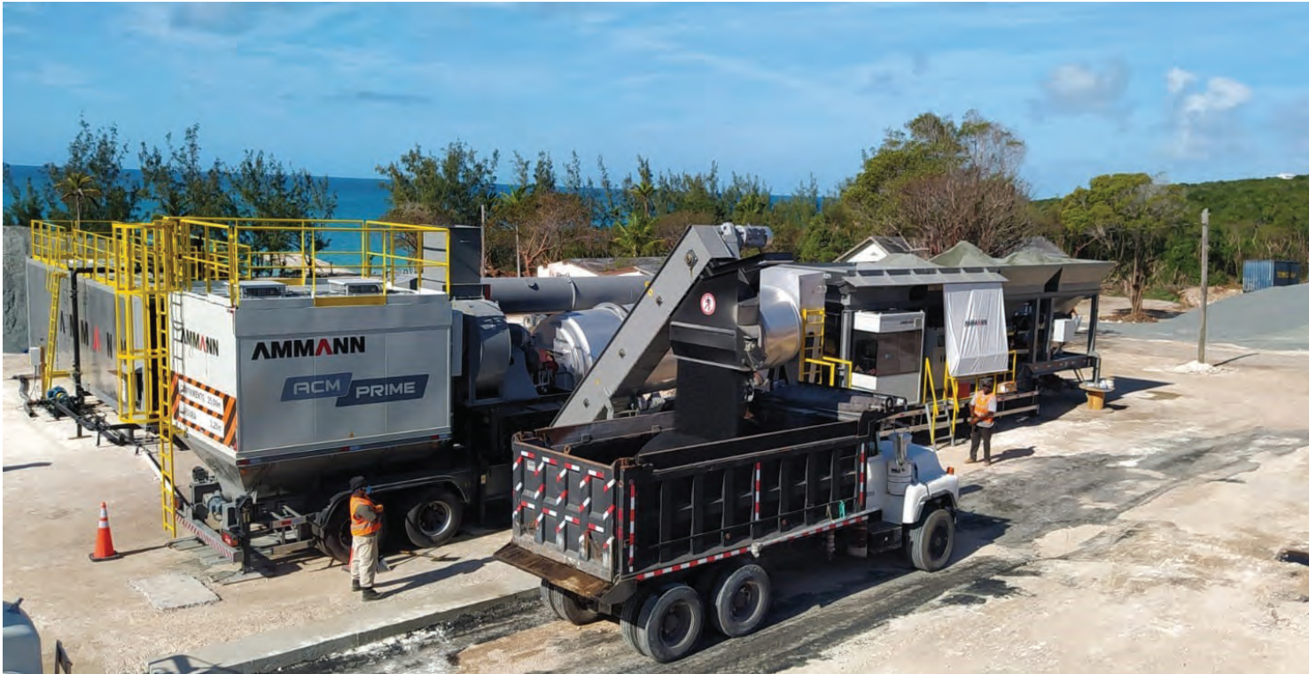
ABOVE: For the project, BHM used an Ammann ACM 140 Prime asphalt batching plant. The unit has a production capacity of 140 tons per hour.
