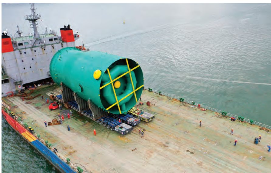
The 1,357-ton regenerator being transported on Goldhofer 3x20 PST/SL axle lines to a refinery project in Balikpapan, East Kalimantan.
