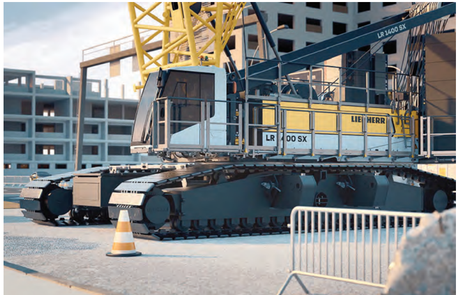
ALL IMAGES: The new Liebherr LR 1400 SX crawler crane has a wide range of applications. With a compact transport weight of 46 t, the machine can be easily relocated between jobsites.
