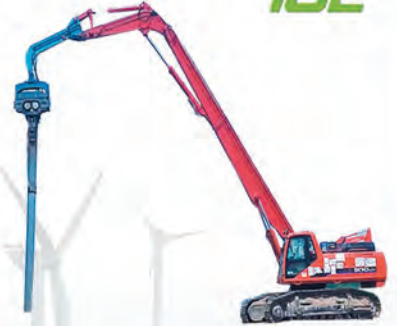
Excavator Vibro Hammer
