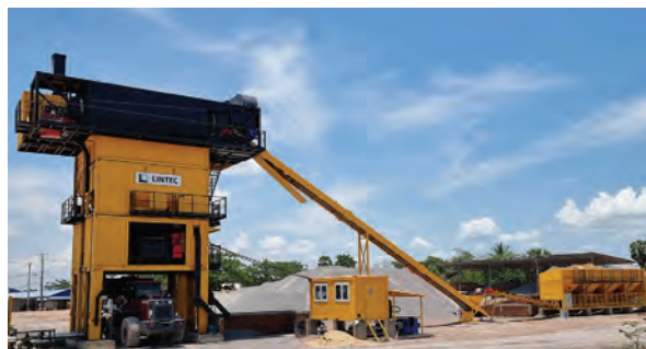
Lintec CSD2500B asphalt plant is built in ISO shipping containers, ensuring economical transportation and fast setup.
